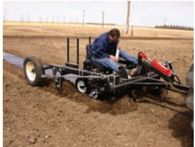
A specialized plastic mulch applicator is necessary to properly install. Life span up to five years; labour intensive if not mechanized.
